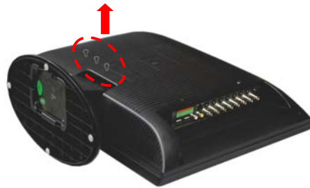
[Fig. 5-4 Removing three screws]
